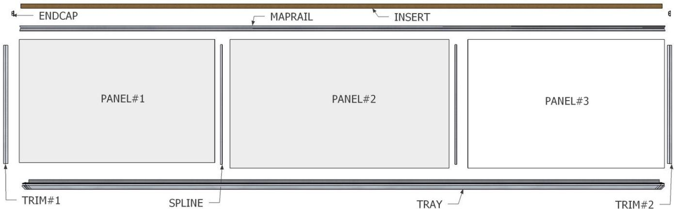
1. Lay out all pieces on floor & match up pieces into configuration. Re-check your order's installation measurements & trim sizes for each location.
